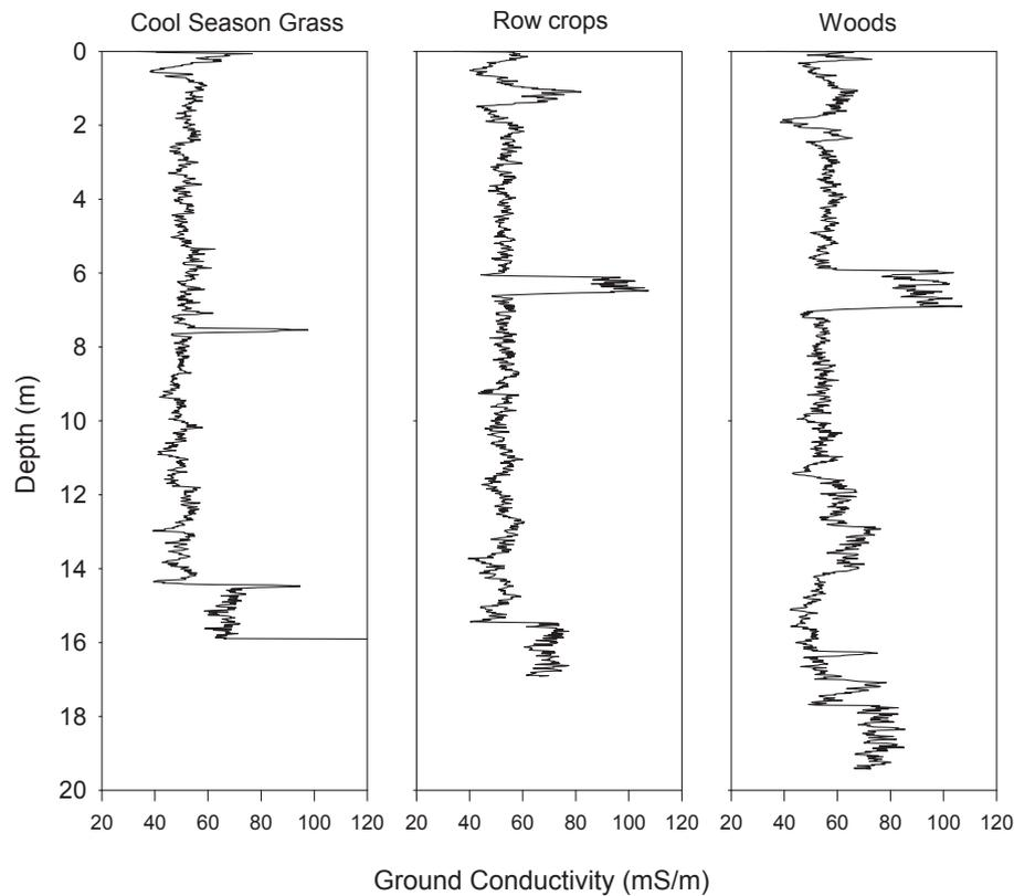
Fig. 2. Borehole geophysical log of ground conductivity measured at the center well of the three land cover sites using the Geoprobe™ hydraulic probe.
