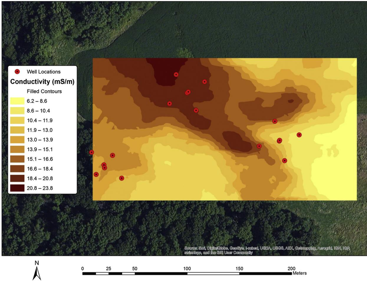
Fig. 3. Ground conductivity measured using surface geophysics (EM-31).
